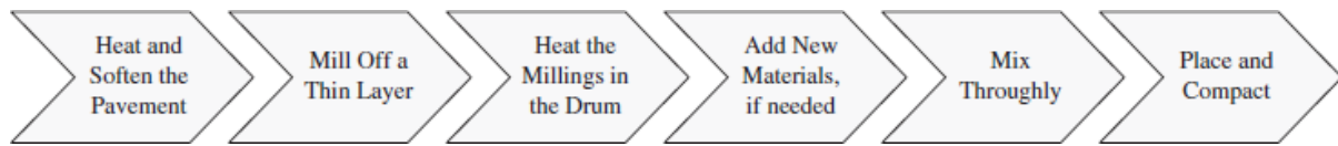
Figure 16 Basic Steps of Hot in-Place Recycling
